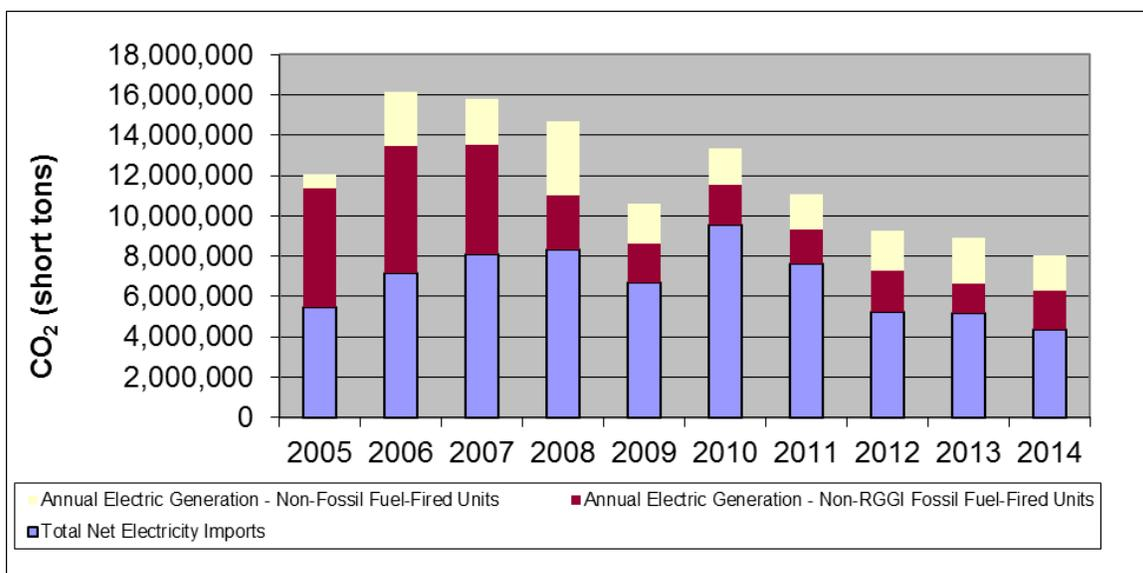
**Figure 17. CO<sub>2</sub> Emissions from Non-RGGI Generation Serving Load in NYISO (short tons CO<sub>2</sub>)**
