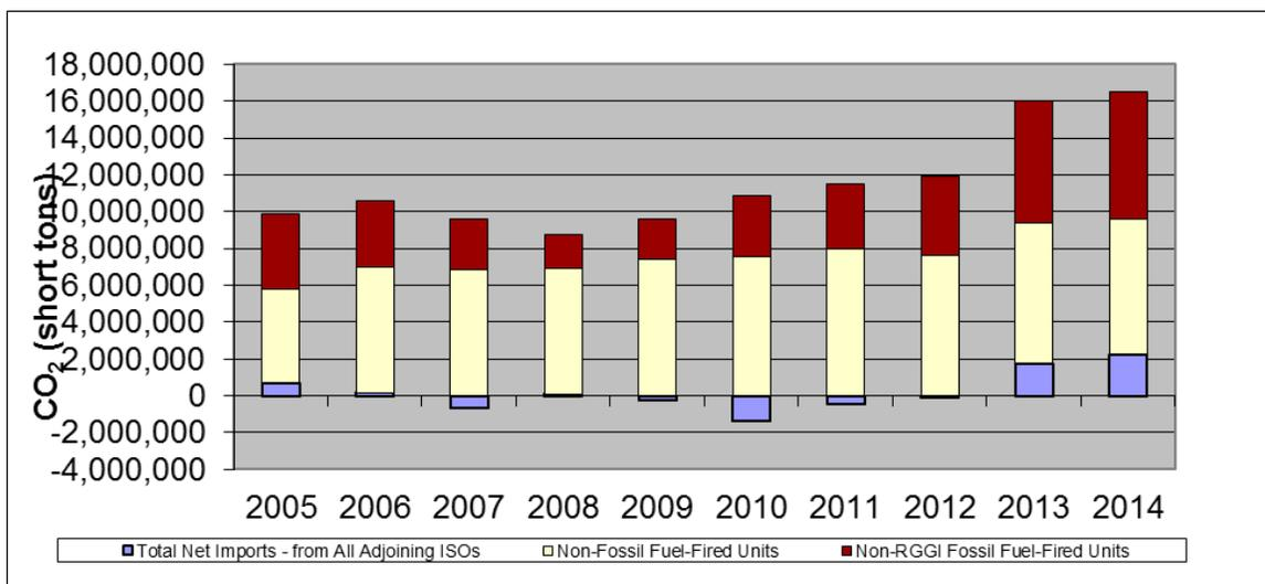
Figure 12. CO<sub>2</sub> Emissions from Non-RGGI Generation Serving Load in ISO-NE (short tons CO<sub>2</sub>)
