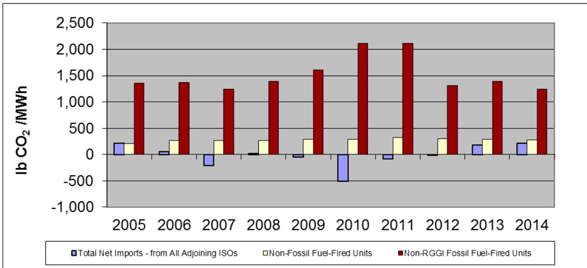
**Figure 13. CO<sub>2</sub> Emission Rate for Non-RGGI Generation Serving Load in ISO-NE (lb CO<sub>2</sub>/MWh)**
